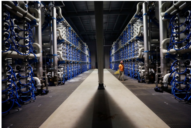
A worker passes rows of tubes used in the reverse osmosis process at the Carlsbad Desalination Project in California on Sept. 22, 2015.(Gregory Bull/AP)
