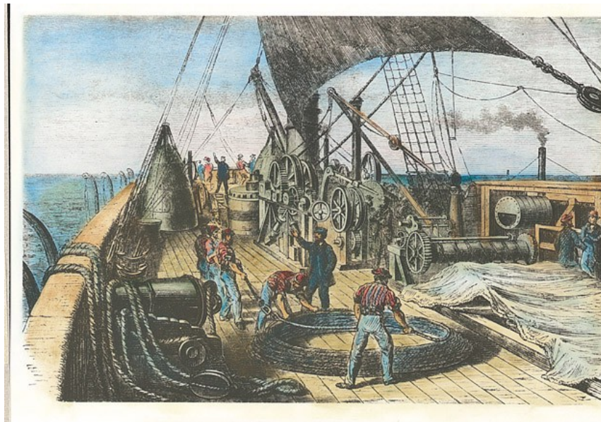
The transatlantic telegraph cable was the first intercontinental communications link of the electric age. This illustration shows the Great Eastern, the largest ship afloat, which laid a permanent cable in 1866.
